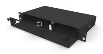
Unloaded 14" modular sliding patch panel for up to 12 ports. Its modularity allows the integration of a wide variety of connector types, and the management of up to 24 fibres within the panel.
