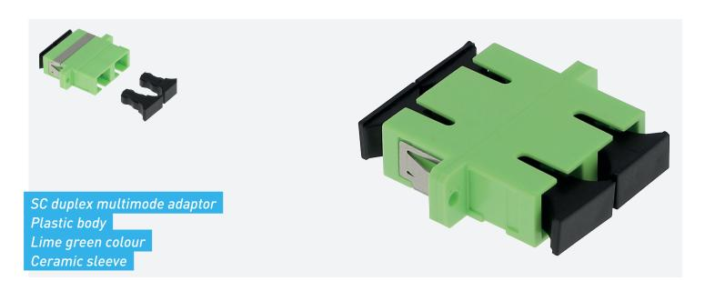
Fiber optic adapters (or bulkheads) allow two fibers equipped with connectors (pre-connectorized optical fibers, patchcords, etc...) to be connected to each other, via a ceramic sleeve.
