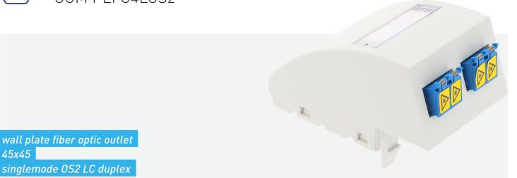
The LC OS2 optical outlet, in a 45 x 45 mm module format, will integrate perfectly on trunking, poles, or GOP boxes in office areas. Equipped with 2 LC duplex adapters and their dust covers, its discreet rounded profile helps to limit the bending of the user patchcord. A label and its protective window facilitate the identification of the optical port.
