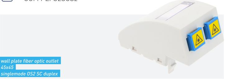
The SC duplex OS2 optical outlet, in a 45 x 45 mm module format, will integrate perfectly on trunking, poles, or GOP boxes in office areas. Equipped with 2 SC simplex adapters and their dust covers, its discreet rounded profile helps to limit the bending of the user patchcord. A label and its protective window facilitate the identification of the optical port.
