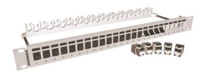
The GIGAMEDIA metal patch panel allows for the use of the 28 mm deep tool less terminated jack to be fitted. The jack can be terminated separate from the patch panel, and easily inserted into the specific port. The keystone jack exceeds all Category 6A performance levels required by standards (see page 12 for
