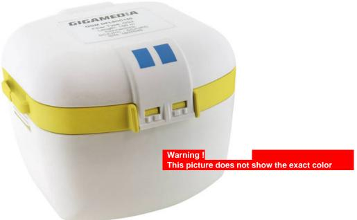
Launch reels are essential during reflectometry tests. Positioned at the start and end of the link, they allow the input and output connectors to be qualified, and eliminate any reflectometer dead zones. With a cube shaped format, they combine practicality, performance and robustness in order to perform the tests easily.
