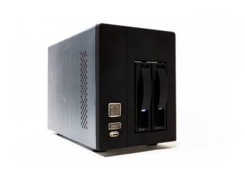
TheNXSERV20L2B is a server based on Windows 10 IoT Entrerprise. It is fully designed to support the performance needed for a CCTV project based on VMS NX Witness from Network optics.
