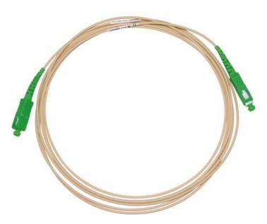
The Gigamedia subscriber patch cords allow the terminal socket to be connected to the internet operator's box. Of small diameter (2mm) and compliant to ITU-T G657A2 specifications (low bending radius cables), they meet the restrictions for residential installations, and in particular may be laid along plinths or around door frames. Available in ivory colour, they easily blend in with the design of both collective and individual housing.
