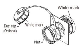
Precaution on secured sealing mating:
