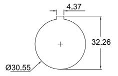
Recommended cutting on panel, panel thickness 0.7 ~ 2.0mm
