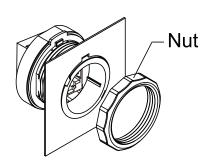
2. Screw the nut to fix the IP68 socket housing on the panel (or your device).
