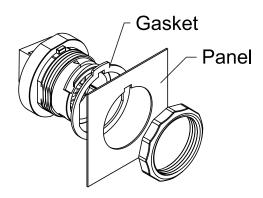
1. Before place the IP68 socket housing to panel (or your device), make sure the gasket is between the panel (or your device) and the housing properly.
