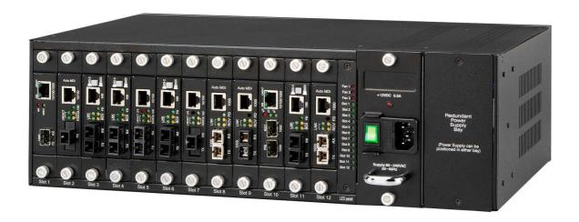
The GGM 719 is a highly engineered product designed to offer a lifetime of operation. Incorporated in the chassis are three long life cooling fans to ensure a cool operating environment. Each fan is monitored and connected to the LED status panel mounted on the front. The LEDs indicates when power is supplied to each module and that the fans are functioning correctly.
