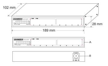
A. Gigabit PoE Injector Ports B. 100-240 VAC, 50/60 Hz
