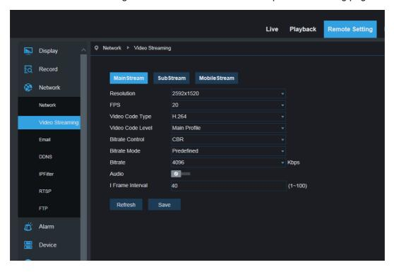
By default the available bit streams are: main bit stream, sub-bit stream and cell phone bit steam.
