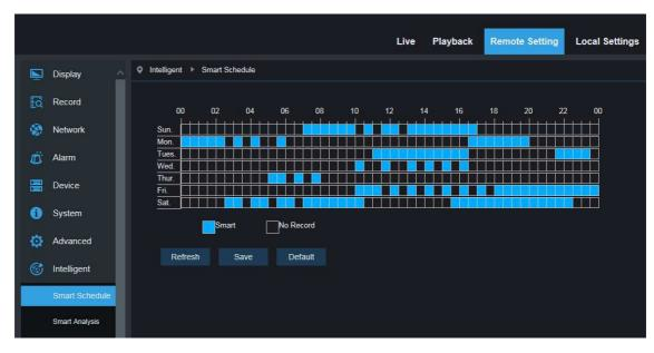
one grid in the table is 30 minute, User can setup according to private requirement to choose different record type and time.
