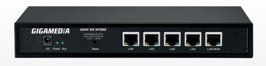
The GGM WCAP100 Wireless Controller is a WLAN controller for wireless AP. It can manage, control and monitor 12 AP in the same networking diagram simultaneous. It makes the small area WiFi solution in the hotel, school, industrial, supermarket, a restaurant more easy in setting, control, and monitoring. And because of the controller, you will save human energy for the maintenance of the whole solution.
