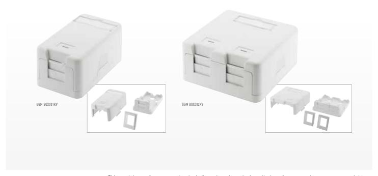
This modular surface-mount box is dedicated to allow the installation of up to two keystone type modules (GGM BOX002KV). It has been designed to make the module replacement easier. This solution allows for quick network modernization without the need to replace the entire box. The box can be mounted on the wall with screws or double-sided self-adhesive foam.
